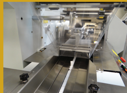
◀ Delicate product conveyor with carrier card in-feed guide rails to handle product transitioning to the custom fixed former.
