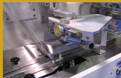
◀ Deluxe Adjustable Former provides an improved film flow, similar to a fixed former while maintaining versatility
